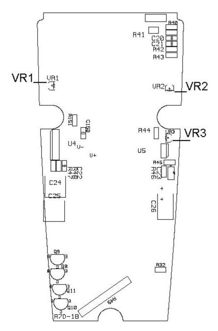
**Figure 3 - Calibration Adjustment Points**
